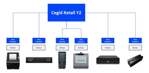
Instead of exchanging directly with each device, the POS terminal communicates with a generic multi-device connector called CPOS.
